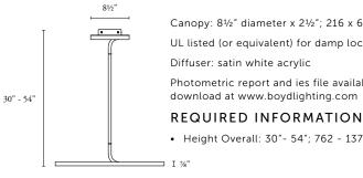
Canopy:  $8\frac{1}{2}$ " diameter x  $2\frac{1}{2}$ "; 216 x 64 mm UL listed (or equivalent) for damp locations
