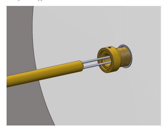
12. Carefully slide fixture arms into the mud collars until they stop, about 1". Secure with the small set screws, using the provided Allen wrench.
