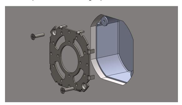
6. Secure the adjustment plates to the mud plates using the large, truss head screws that were provided. The large holes allow the adjustment plates to be slid upward/downward, and laterally. Check to make sure the center-to-center distance of the shaft corresponds to the distance listed on the Step 1 Chart. Check to make sure that the shafts are level with one another.
