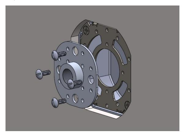
7. With the screws on the adjustment plates fully tightened, prepare for mudding work.
