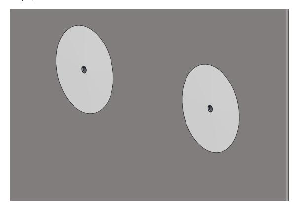
9. The mudded-over shaft should protrude slightly from the mud, or be flush. Take precautions to make sure that the hole and threads remain free of mud.
