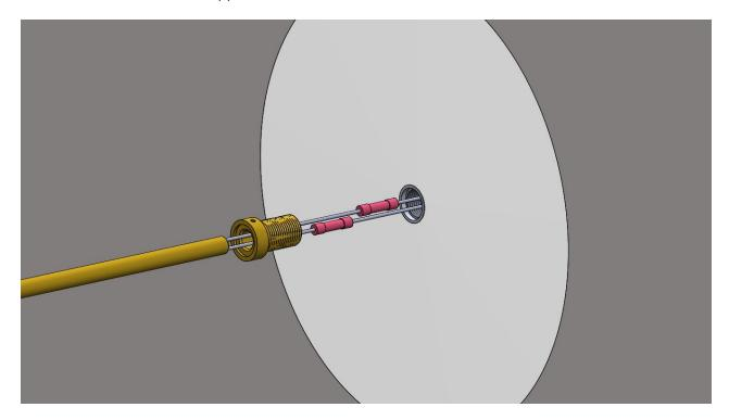
11. After crimping, carefully thread the brass mud collar directly into the wall shaft until fully tightened. Repeat this step on the opposite side.
