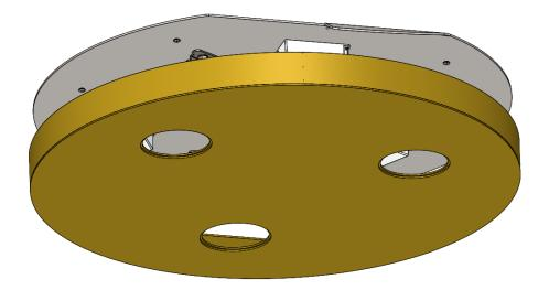
5. Begin assembly of the shade assemblies. Slide the wired heatsink through the bottom of the slender, inner glass shade. Gently pull wiring out the top hole.
