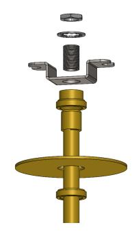
9. With main stem and shade assembled, carefully lift assembly near canopy hole.
