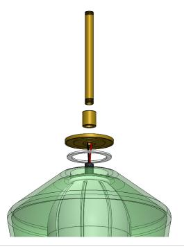
8. At top of stem, place the swivel aligner. Unthread the collar on the swivel so it drops down on the stem. Slide thin disk over stem. Secure hang bracket to top of stem using a nipple, lock washer, and nut. Wiring not shown.
