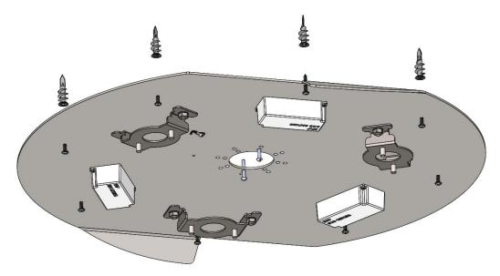
3. With ceiling mount disk affixed to the ceiling, make wire connections. Connect white driver wire to ceiling neutral wire (typically white). Connect the black driver wire to ceiling hot wire (typically black). Connect ground wire to ceiling ground wire or screw. For those using 0-10V dimming, connect the purple and pink wires to the ceiling dimming wires (purple/pink). For basic phase-dimming on an ELV or Triac style dimmer, simply cap off the purple and pink wires which need not be used.
